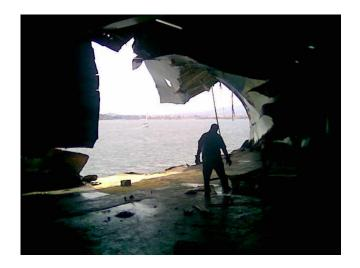
On 21<sup>st</sup> June 2006, in dense fog suddenly materialising at sea in the vicinity of the port entrance in Olbia (Sardinia), passenger ro/ro "Nuraghes" collided with passengers ro/ro "Moby Fantasy". The collision caused a long breach in the hull of "Nuraghes" (about 30 mt. length). Conversely the fore of the "Moby Fantasy" was heavily damaged with ingress of water which did require immediate assistance by part of tugs. Both vessels entered Olbia port where they were safely moored.
