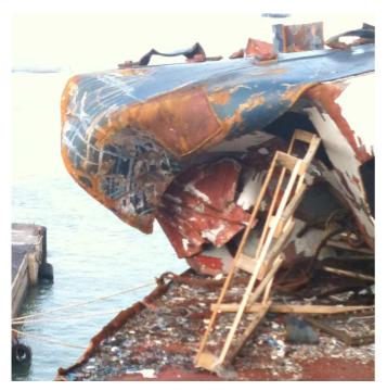
On 17<sup>th</sup> December 2010, the ro-ro vessel "Delfino Bianco" collided with the ferryboat "Moby Wonder" during night navigation between Marina di Carrara and Olbia, in the open sea close to Isola d'Elba. The collision caused a long rip along the right side of the ferryboat "Moby Wonder" and to the bow and the left side of the vessel "Delfino Bianco".
